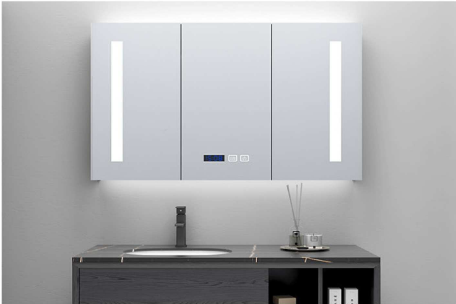
SVMC007 Dimension: 24*36*5" (610*914*127mm) or customized Mirror: 3/4/5mm Copper Free Silver Mirror Switch: Touch/motion sensor/or no switch Light source: LED SMD 2835, 120 or 60pcs/m Color Temperature: 3000K, 4000K, 6000K ICRI: > 90 Voltage: AC 110~240V, 50/60Hz
