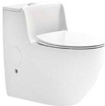
SV2063 One-Piece Toilet Flushing System: Washdown Size: 650x360x600mm P-trap: 180mm S-trap: 300/400mm
