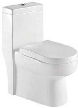
SV2017 One-Piece Toilet Flushing System: 2 Super Siphonic Size: 650x350x740mm S-trap: 220/300/400mm
