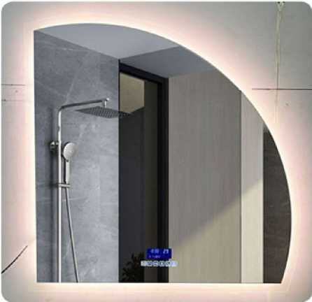
SVBM004 Dimension: 24*36" (610*914mm) or customized Mirror: 3/4/5mm Copper Free Silver Mirror Switch: Touch/motion sensor/or no switch Light source: LED SMD 2835, 120 or 60pcs/m Color Temperature: 3000K, 4000K, 6000K ICRI: > 90 Voltage: AC 110~240V, 50/60Hz
