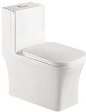
SV2012 One-Piece Toilet Flushing System: Siphonic Size: 670x375x745mm S-trap: 100/200/250/300mm
